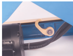
Hinged maintenance catches
