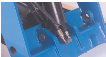
Flow limiting valve provides a controlled descent in the event of a hydraulic line rupture
