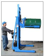
Release the clamp, then raise your drum to place it on a rack up to 8.5' (2.59 m) high on a 4-tier rack.
